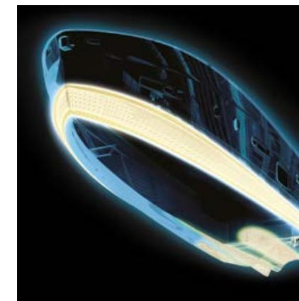
Dual Mode semi-planing hull with a tunnel, skeg and vertical bow (Magellano Collection)
